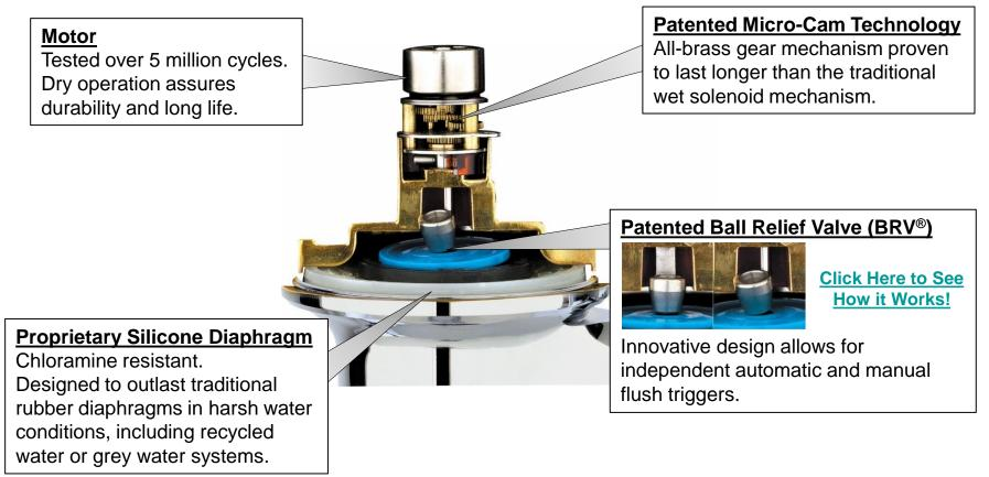
Micro-Cam Technology vs Solenoid
