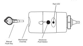
Red LED - Constant blinking red LED indicates batteries are low and need replacing.
