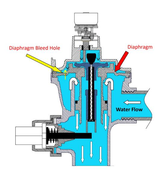
Diaphragm is pushed upward by water pressure and water flushes down the outlet bore.
