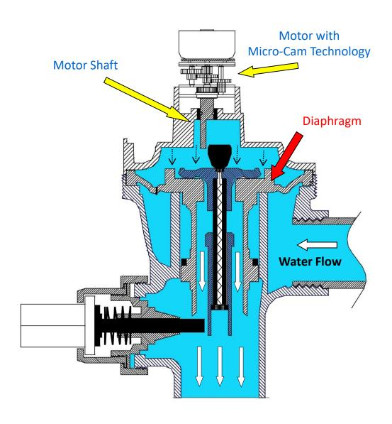
Motor shaft rotates back to closed position.
