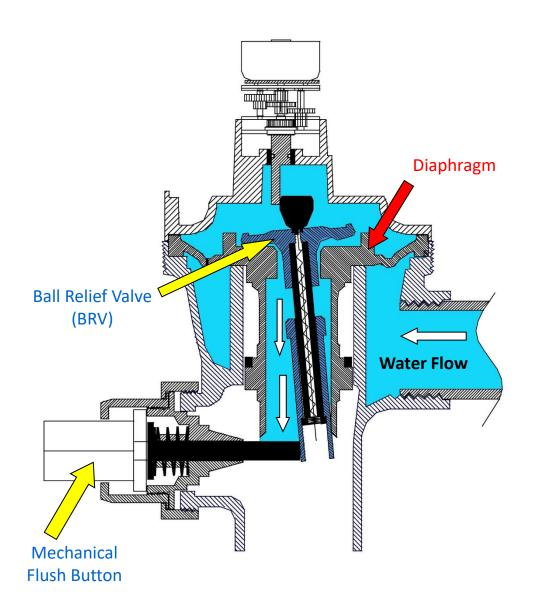
Flush button is pressed, triggering the Ball Relief Valve (BRV) to open position.
