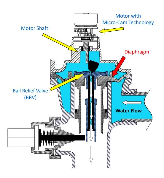
Motor shaft rotates, triggering the Ball Relief Valve (BRV) to open position.
